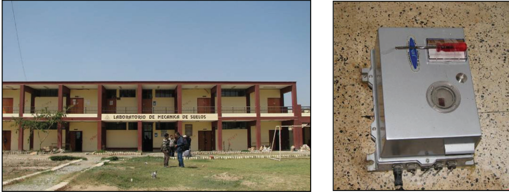
Figure 7.2 ICA2 station with analog accelerometer
