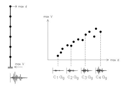
Figure 3.8 Implementation of the incremental dynamic analysis technique (IDA)
