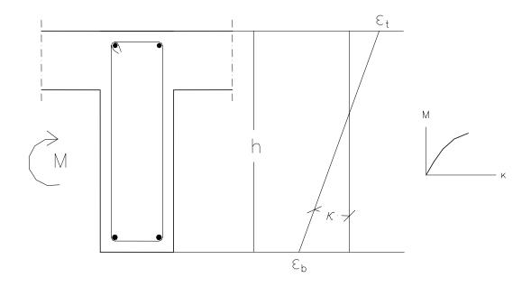
Figure 3.16 Element moment versus section curvature monitoring
