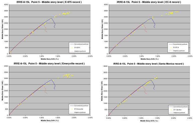
Figure 4.27 Response at the middle story level, irregular structure (low ductility)
