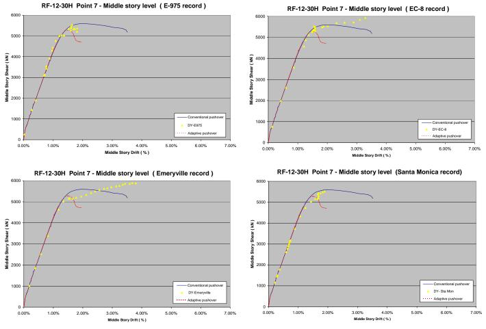
Figure 4.5 Response at the middle story level, regular structure ( high ductility )
