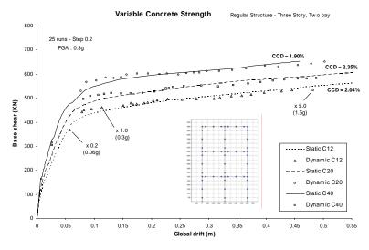
Figure 3.18 Application of the Capacity Curve Discrepancy Factor (CCDF)
