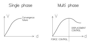
Figure 2.6 Single versus multi-phase solution
