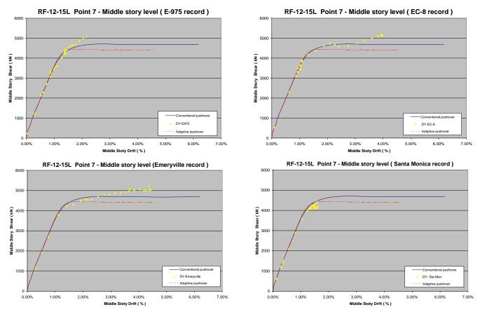
Figure 4.6 Response at the middle story level, regular structure (low ductility)
