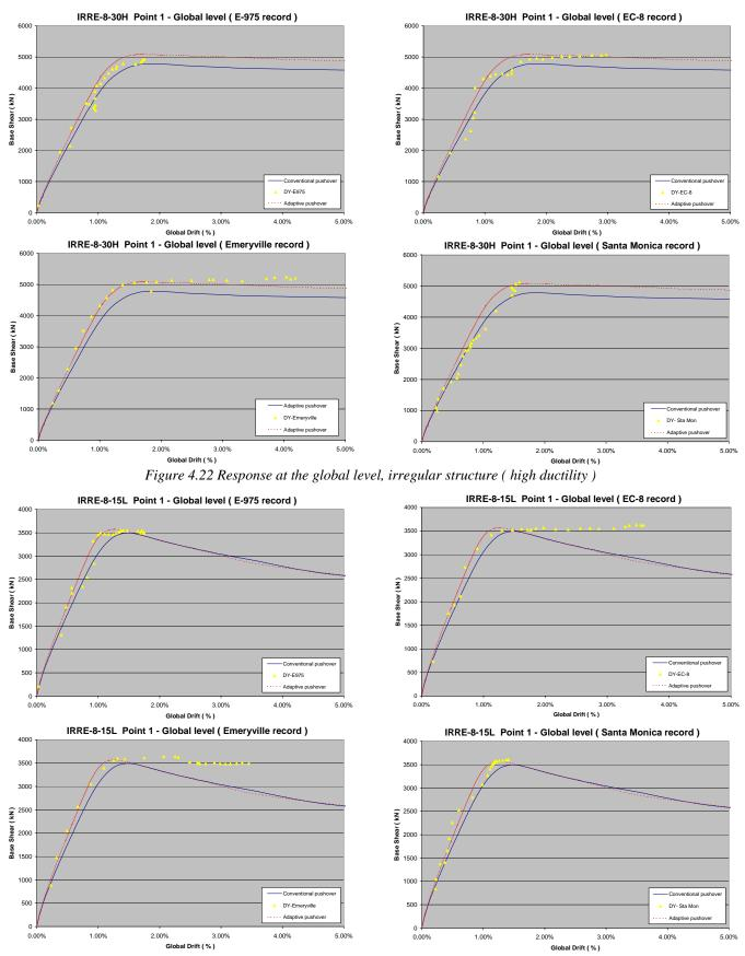
Figure 4.23 Response at the global level, irregular structure (low ductility)
