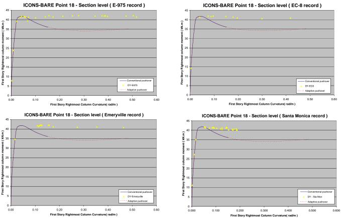
Figure 4.36 Response at the section level, ICONS bare frame
