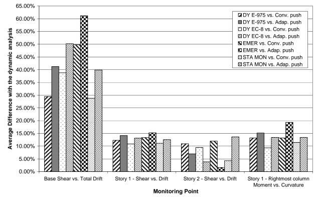
SPEAR 3D-FRAME - Capacity curve discrepancy factors ( CCDF )
