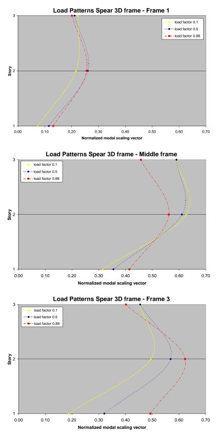
Figure 4.41 Variation on the modal scaling vector, for different load factors in the SPEAR building frames.
