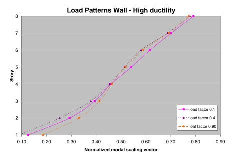
Figure 4.17 Variation on the modal scaling vector, for different load factors.
