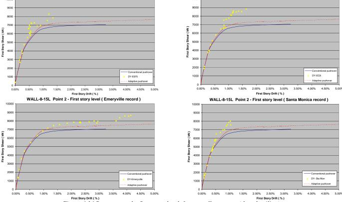
Figure 4.14 Response at the first story level, frame-wall structure ( low ductility )
