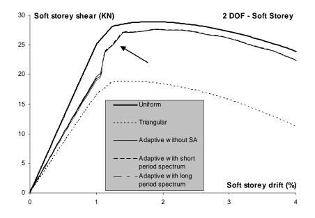
Figure 2.10 Story shear versus drift plot for the soft story
