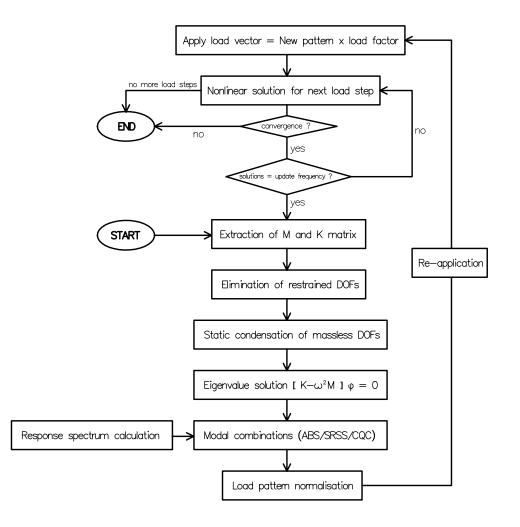
Figure 2.5 Flow chart of the adaptive pushover method
