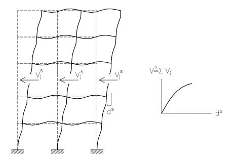
Figure 3.15 Story shear versus interstory drift monitoring
