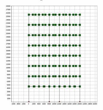
2D reinforced concrete frame with irregularity in elevation.
