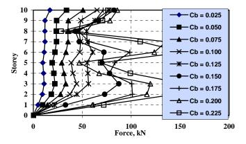
Figure 2.3 Adaptive pushover using story forces to update the lateral load pattern
