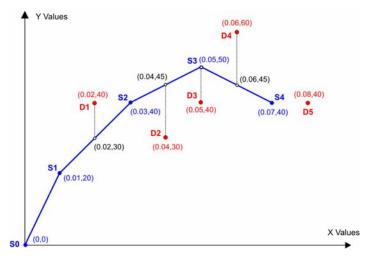
Figure 3.17 Definition of the Capacity Curve Discrepancy Factor (CCDF)
