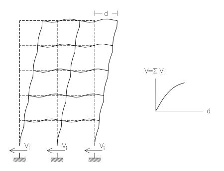
Figure 3.14 Base shear versus global drift monitoring
