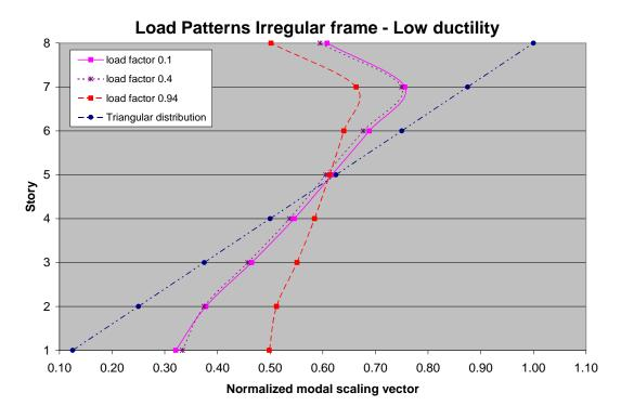
Figure 4.28 Variation on the modal scaling vector, for different load factors.
