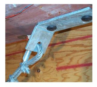
Figure 7.35 Bent plate connection during test - notice crack at bend in plate.
