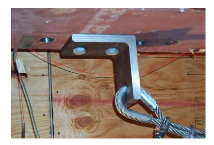
Figure 7.47 L8x8x1" steel angle used in retrofit modification 3 on model bridge.
