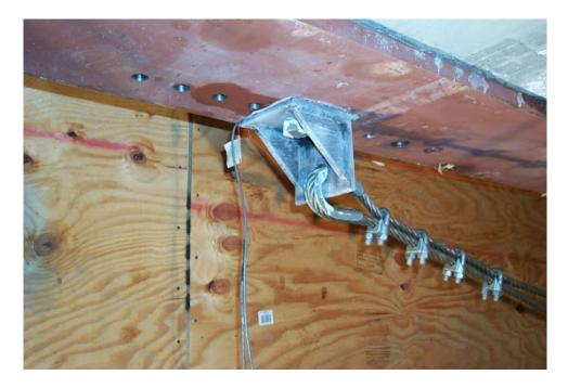
Figure 7.52 Stiffened L6x6x1/2" angle used in retrofit modification 4 on model bridge.
