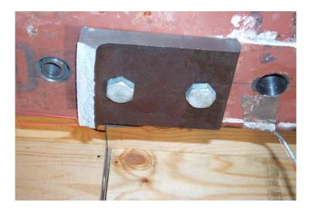
Figure 7.60 Brittle failure of L8x8x1" steel angle tested in retrofit modification 5.
