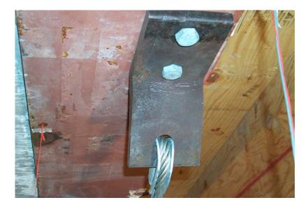
Figure 7.50 Girder connection during testing with cracks forming in k-zone.
