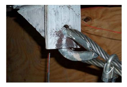
Figure 7.54 Stiffened steel angle girder connection tested in retrofit modification 4.
