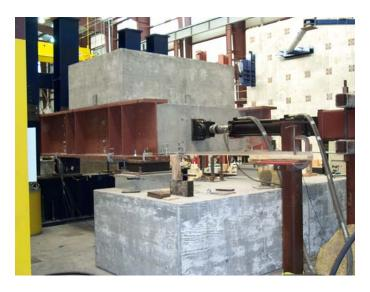
Figure 7.8 Two concrete blocks representing the dead weight of the bridge.
