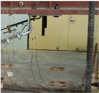
Figure 7.33 Bent plate girder connection tested on model bridge.
