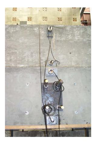
Figure 7.18 Seismic accelerometers mounted at top and bottom of dead weight blocks.
