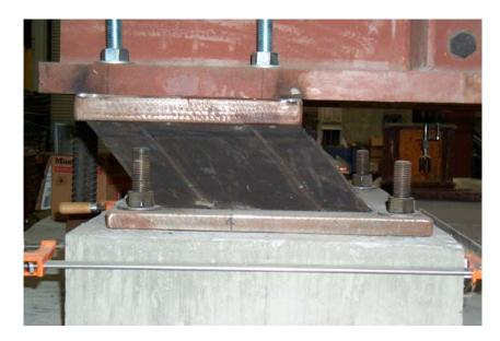
Figure 7.25 Bearing displaced to 100% shear strain.
