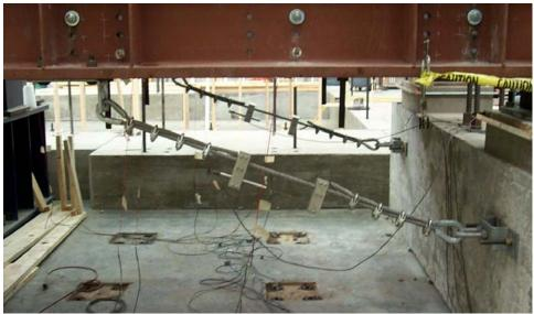
(b) Connection between Deck and Abutment or Pier
