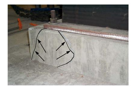
Figure 7.26 Cracks formed in concrete pedestal after bearing was subjected to 100% shear strain.
