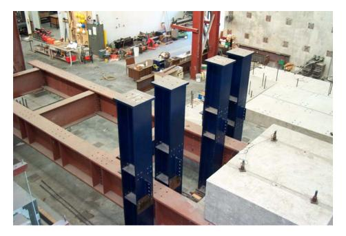
Figure 7.11 Columns used to restrict out-plane-movent.
