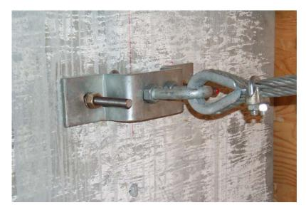
Figure 7.32 Bent plate pier connection tested on model bridge.
