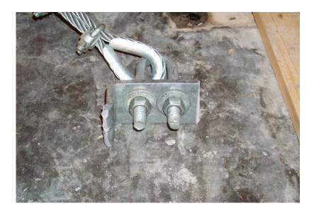
Figure 7.39 Bent plate pier connection failure after test retrofit modification 1.
