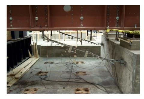
Figure 7.14 Cable restrainers were attached between girder flange and pier.
