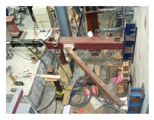
Figure 7.12 Actuator extender tube and connection elements to the reaction wall.
