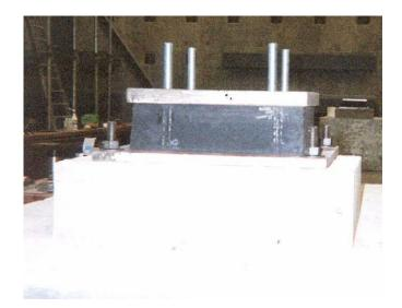
Figure 7.7 Elastomeric bearing assembly.
