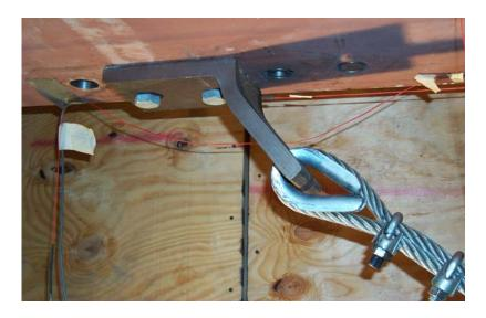
Figure 7.49 L8x8x1" steel angle connection used tested in retrofit modification 3.
