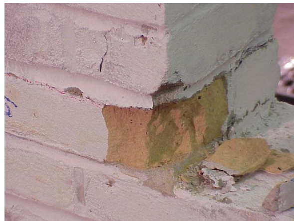
c) NE Brick Cracking at 2.5% Drift
