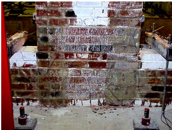
b) Delamination Pattern of SE FRP Strip
