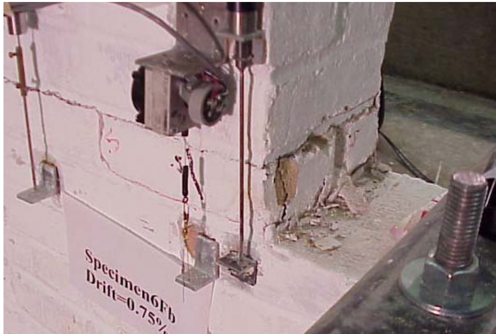
a) SW Toe Compression Splitting
