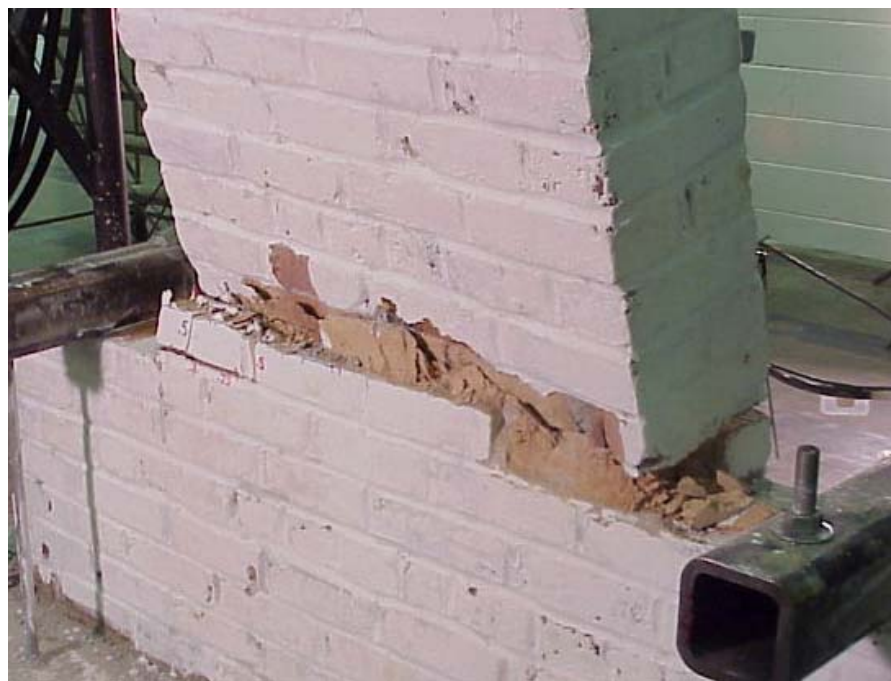
b) Toe Crushing at 1.5% Drift
