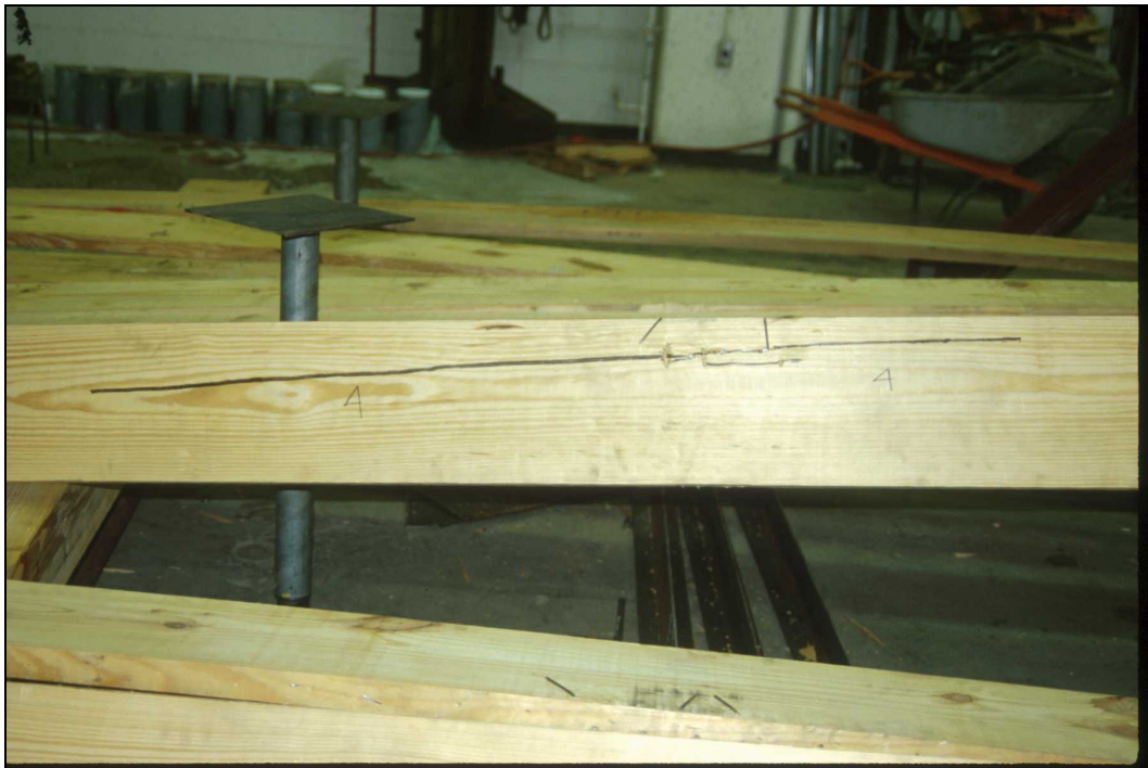
FIG. 4.20 Crack in Joist of Diaphragm MAE-1B (After Disassembly)
