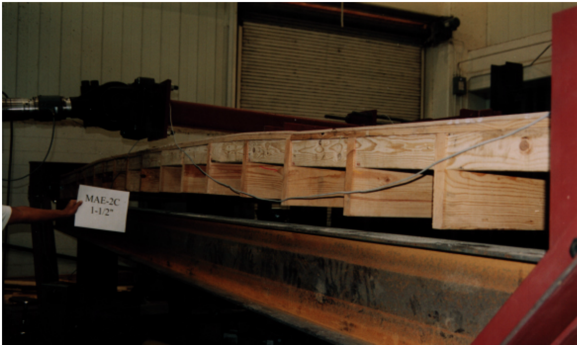
FIG. 4.46 Uplifting of Diaphragm MAE-2C at 38 mm (1.5 in.) of Applied Displacement
