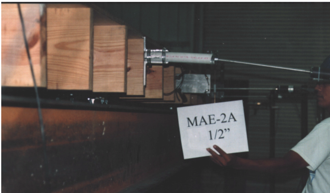
FIG. 4.32 Uplifting of Diaphragm MAE-2A at 13 mm of Applied Displacement
