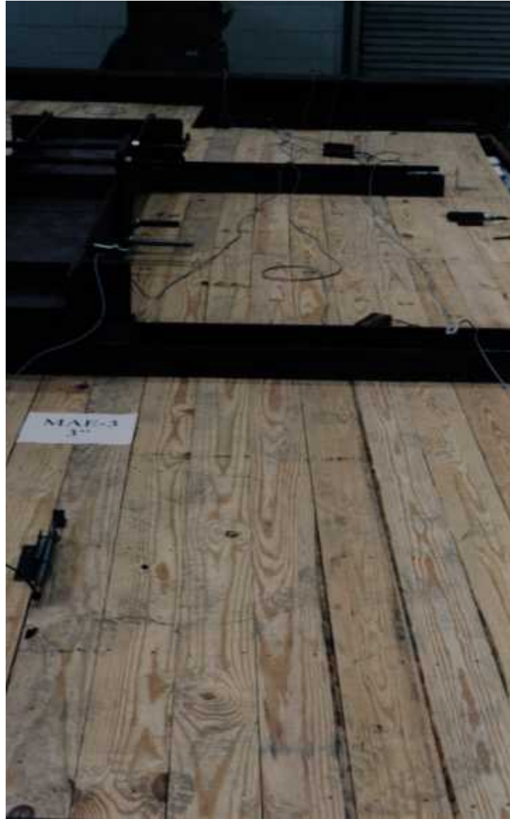
FIG. 4.53 Diaphragm MAE-3 at 76 mm (3 in.) of Applied Displacement
