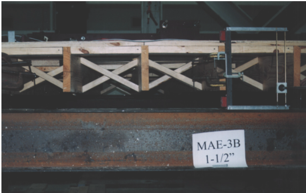
FIG. 4.66 Uplifting of Diaphragm MAE-3B at 38 mm
